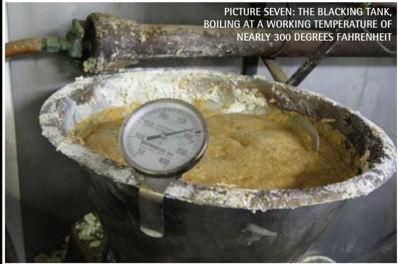
PICTURE SEVEN: THE BLACKING TANK, BOILING AT A WORKING TEMPERATURE OF NEARLY 300 DEGREES FAHRENHEIT
