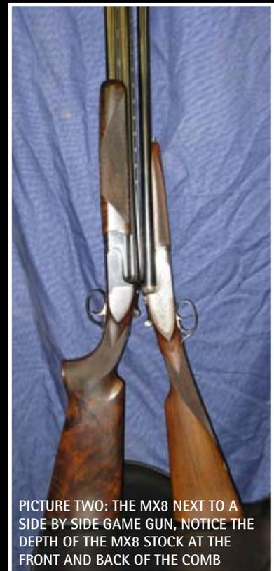
PICTURE TWO: THE MX8 NEXT TO A SIDE BY SIDE GAME GUN, NOTICE THE DEPTH OF THE MX8 STOCK AT THE FRONT AND BACK OF THE COMB
