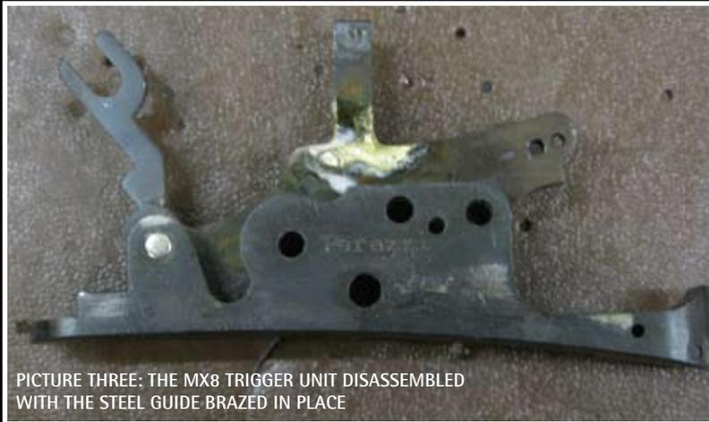
PICTURE THREE: THE MX8 TRIGGER UNIT DISASSEMBLED WITH THE STEEL GUIDE BRAZED IN PLACE
