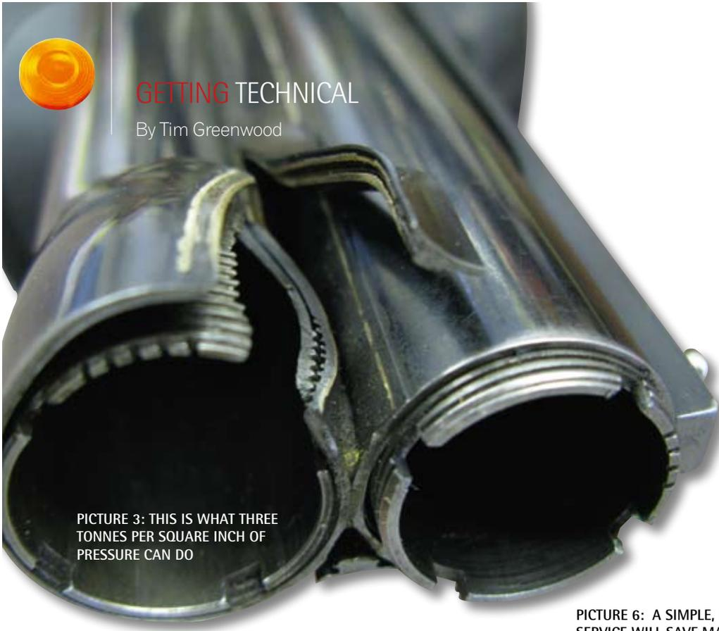
PICTURE 3: THIS IS WHAT THREE TONNES PER SQUARE INCH OF PRESSURE CAN DO
