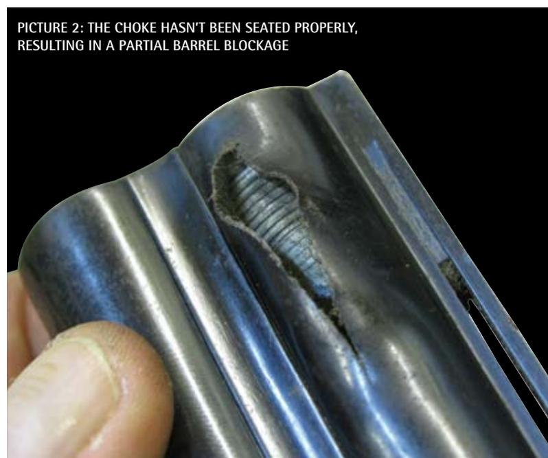
PICTURE 2: THE CHOKE HASN'T BEEN SEATED PROPERLY, RESULTING IN A PARTIAL BARREL BLOCKAGE
