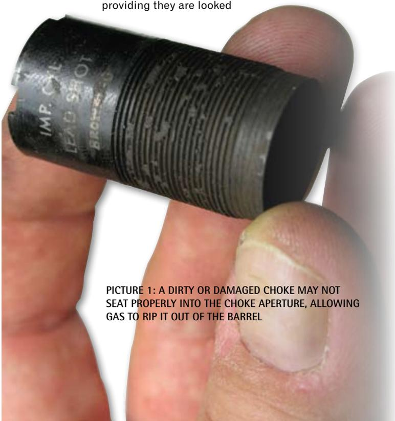
PICTURE 1: A DIRTY OR DAMAGED CHOKE MAY NOT SEAT PROPERLY INTO THE CHOKE APERTURE, ALLOWING GAS TO RIP IT OUT OF THE BARREL
