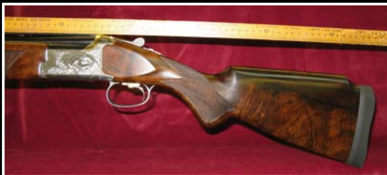
PICTURE 8: FINISHED ARTICLE – THE COMB IS NEARLY PARALLEL TO THE RIB, THE RESULT OF THE SMALL MONTECARLO IN THE COMB, AND THE GRIP A SEMI PRINCE OF WALES
