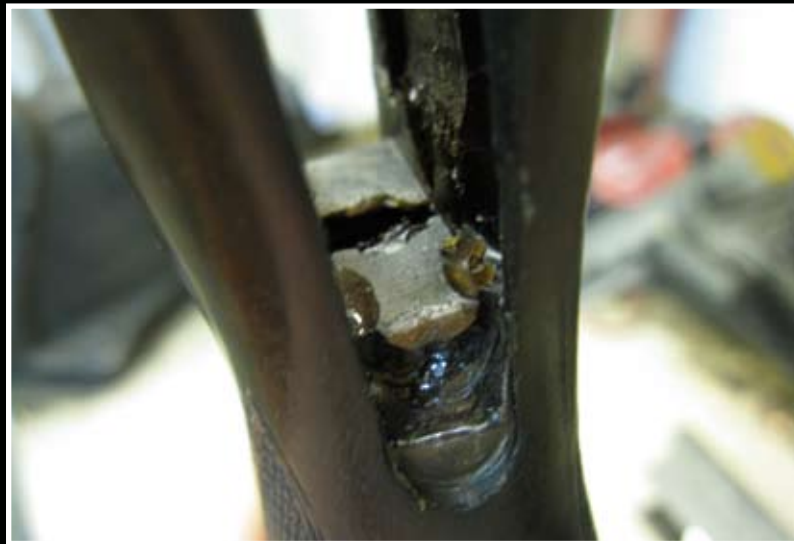
PICTURE 6: THE HEAD OF THE STOCK HAD BEEN BADLY BROKEN SO THE STOCK WAS CUT FROM THE NOSE OF THE COMB TO THE BUTT AND A PIECE OF WALNUT WEDGE INSERTED
