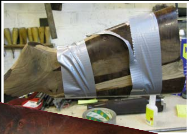
PICTURE 7 (RIGHT) : WORK IN PROGRESS – TRACY WANTED THE SIZE OF THE GRIP REDUCED, AS SHE HAS SMALL HANDS, AND THE GRIP MADE MORE ELEGANT
