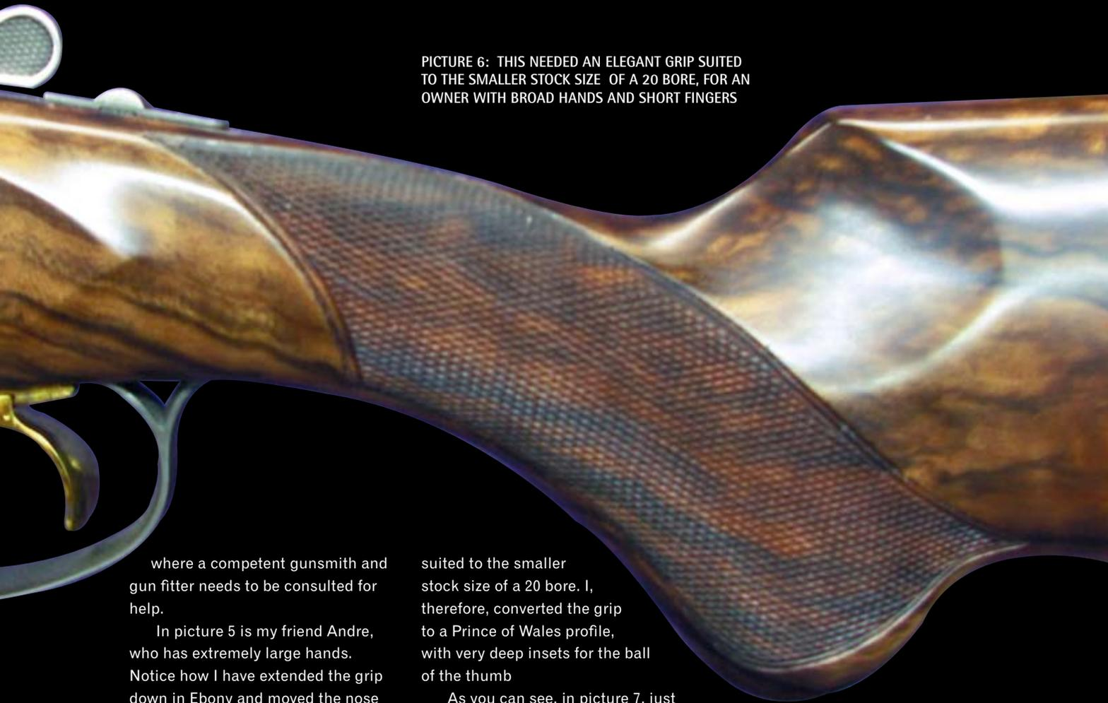
PICTURE 6: THIS NEEDED AN ELEGANT GRIP SUITED TO THE SMALLER STOCK SIZE OF A 20 BORE, FOR AN OWNER WITH BROAD HANDS AND SHORT FINGERS
