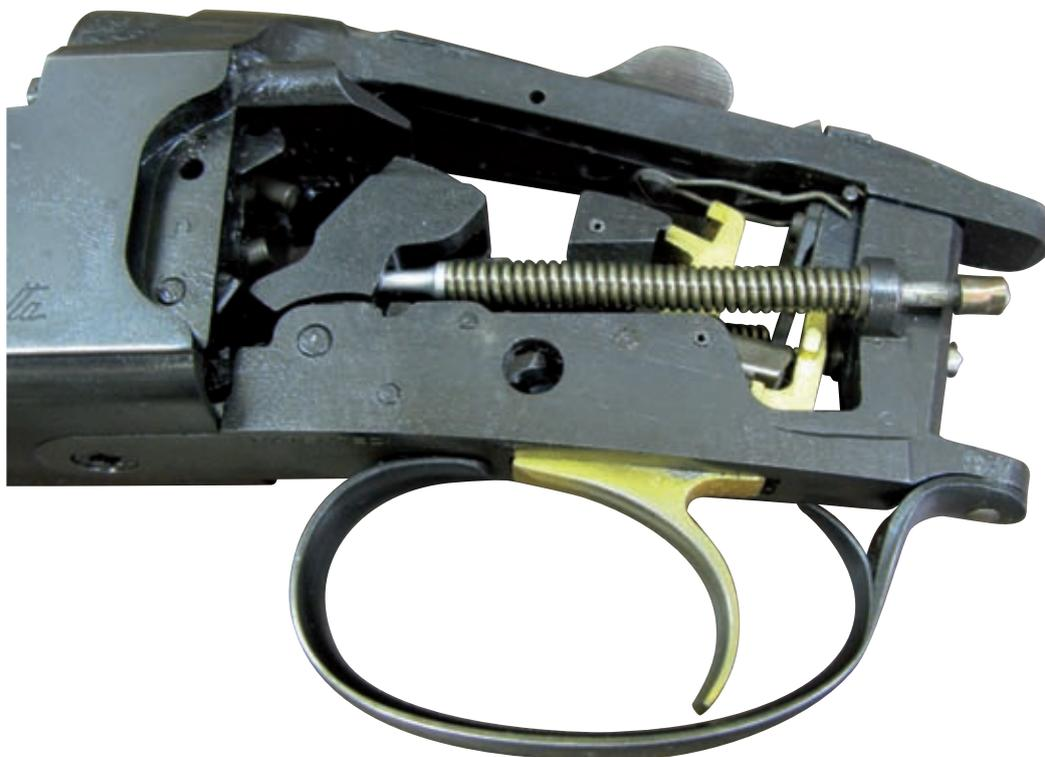
Fortunately they are both very well made guns and straightforward to de-rust. Notice they both now have a smear of grease at the vulnerable points in the action, to prevent wear and water ingress, and a light film of oil applied for protection
