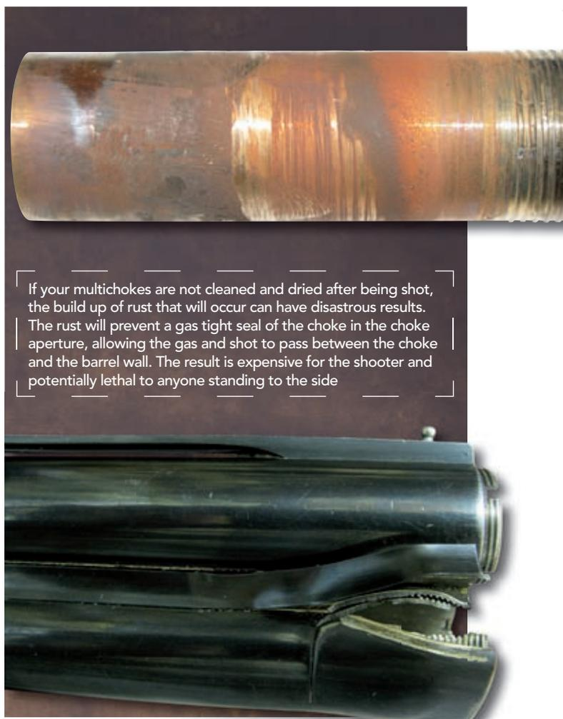
If your multichokes are not cleaned and dried after being shot, the build up of rust that will occur can have disastrous results. The rust will prevent a gas tight seal of the choke in the choke aperture, allowing the gas and shot to pass between the choke and the barrel wall. The result is expensive for the shooter and potentially lethal to anyone standing to the side
