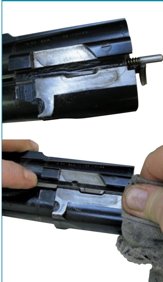
Re-lubricate with light grease; I always use a syringe for this job filled with LM grease available from Halfords, but any good quality grease will do leaving a film in the ejector recess.
