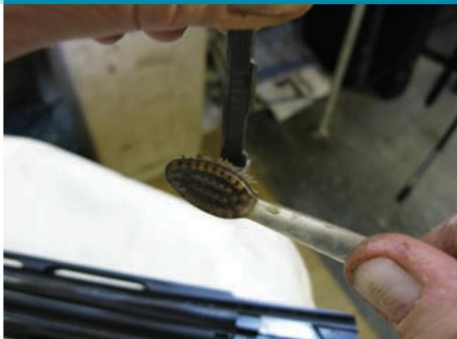
Re-fit the ejector spring and guide. Re-fit the ejector by placing the top edge underneath the top lip of the recess, then compress the ejector against the ejector spring until the lug lines up with the cut out. Twist anti-clockwise until the lug is fully inside the recess then release the pressure on the ejector gradually until it returns to its normal extended position. Repeat this for the other side.
