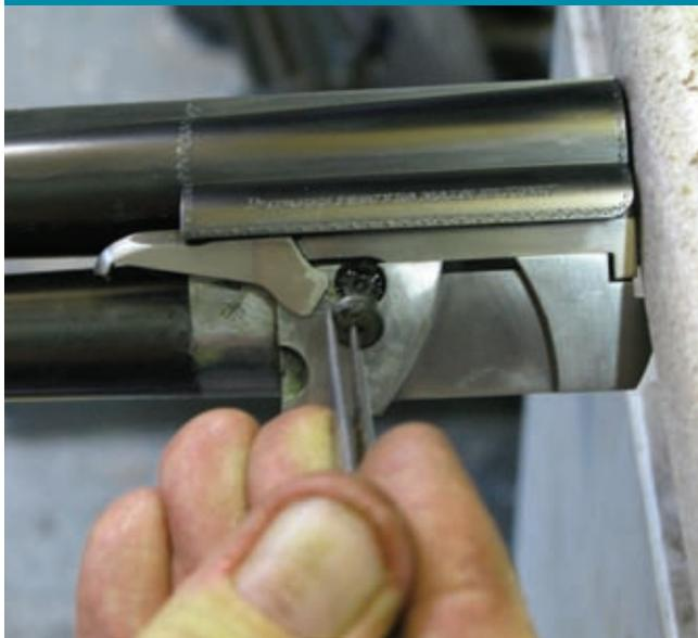
Turn the barrel back over and withdraw the ejector. Once again it is ready for cleaning and re-lubricating. The ejector springs in this case are in the forend and should have a squirt of light oil, but do remove any excess or the forend wood may become soaked in oil and split.
