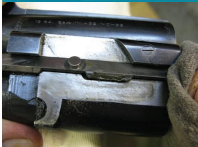
Gently release the pressure on the ejector and it will slide forward away from the breach face. Lift the ejector away and remove the ejector spring guide and the ejector spring.
