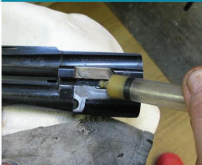
If you are feeling particularly adventurous you can also remove your stock using the stock key provided and give the inside of the action a light spray with oil, but ensure that it is a light spray; do not soak the action then put it back into the stock or the excess oil will be soaked up by the wood and cause even more problems later on. As with the forend, it can over a period
