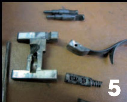
of strain on the locking mechanism as the locking bolt hits the end of its travel without being slowed at all by the chamfer of the barrel lugs mating with it. The small stub which engages with the locking bar at the end of the top lever shaft receives almost a 'kick back' from the pressure of the top lever spring driving the locking bar home via the stub and the shaft with no resistance at the end of its travel. In some cases, this
